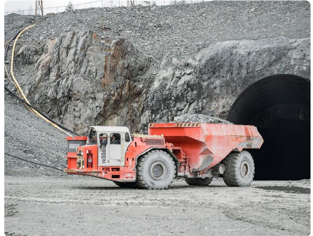
The Lamaque Complex operated two Sandvik TH550B battery electric haul trucks during the year. As of 2026, Eldorado has the largest Sandvik BEV fleet in the industry.
