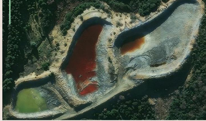
Removal of 500,000 tons of arsenopyrites and contaminated soils and rehabilitation of the original terrain with soil cover and installation of vegetation
