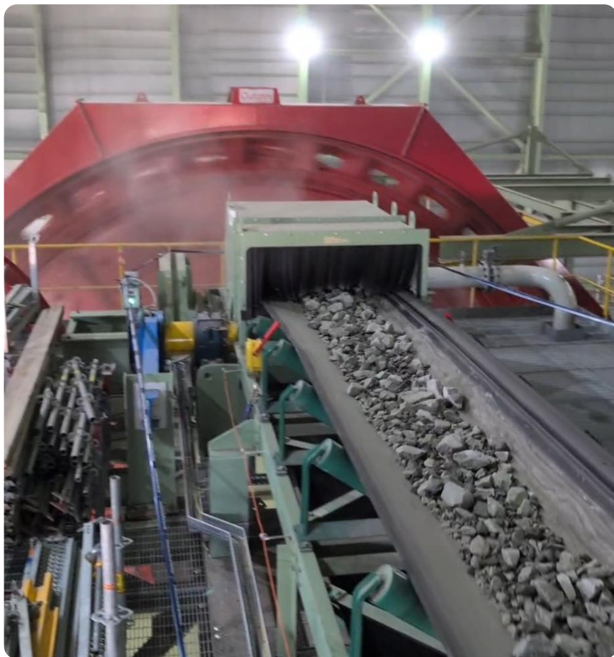
Feeding ore to SAG Mill
