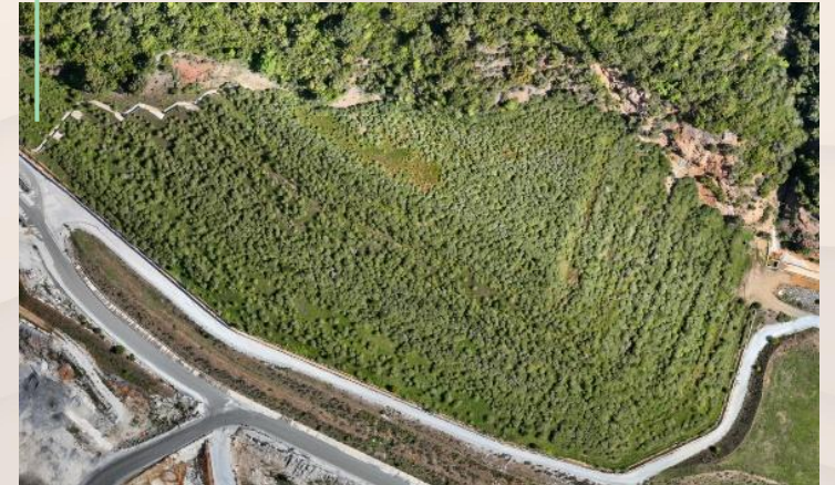
Removal of waste rock, landscaping and hydroseeding.
