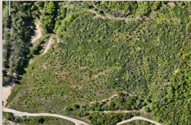
Removal of 500,000 tons of arsenopyrites and contaminated soils and rehabilitation of the original terrain with soil cover and installation of vegetation
