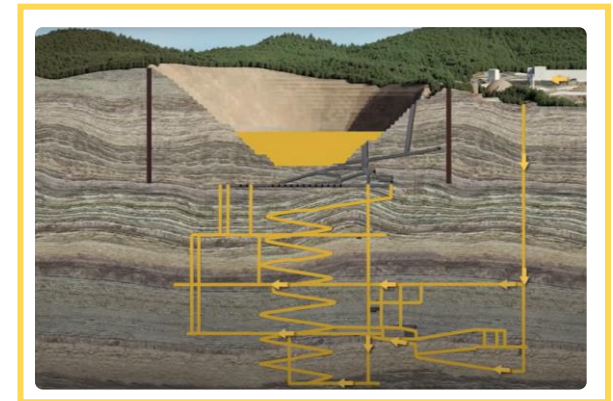
Tailings used as paste back-fill
