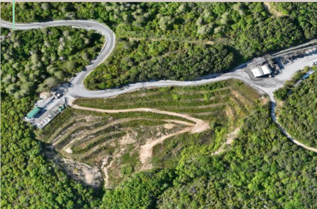
Removal and re-use of 500,000 tons of old mine waste rock as construction materials for the Kokkinolakkas Disposal Facility
