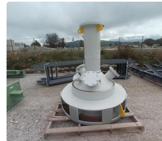
Thickener discharge cone
