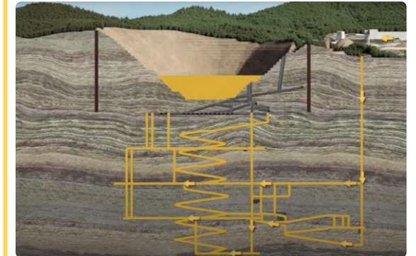
Tailings used as paste back-fill
