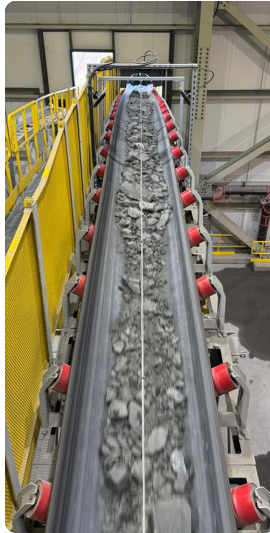
Ore feed to the SAG mill
