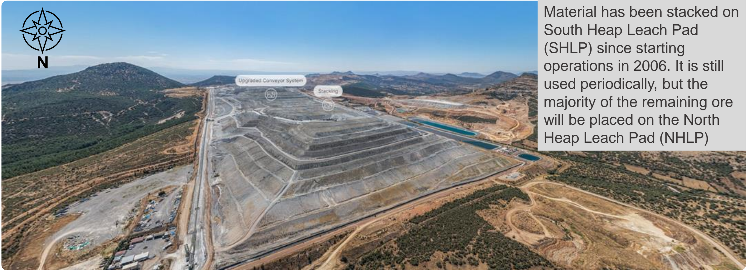
Northern end of the South Heap Leach Pad, showing overland conveyor to the east and process solution ponds to the west
