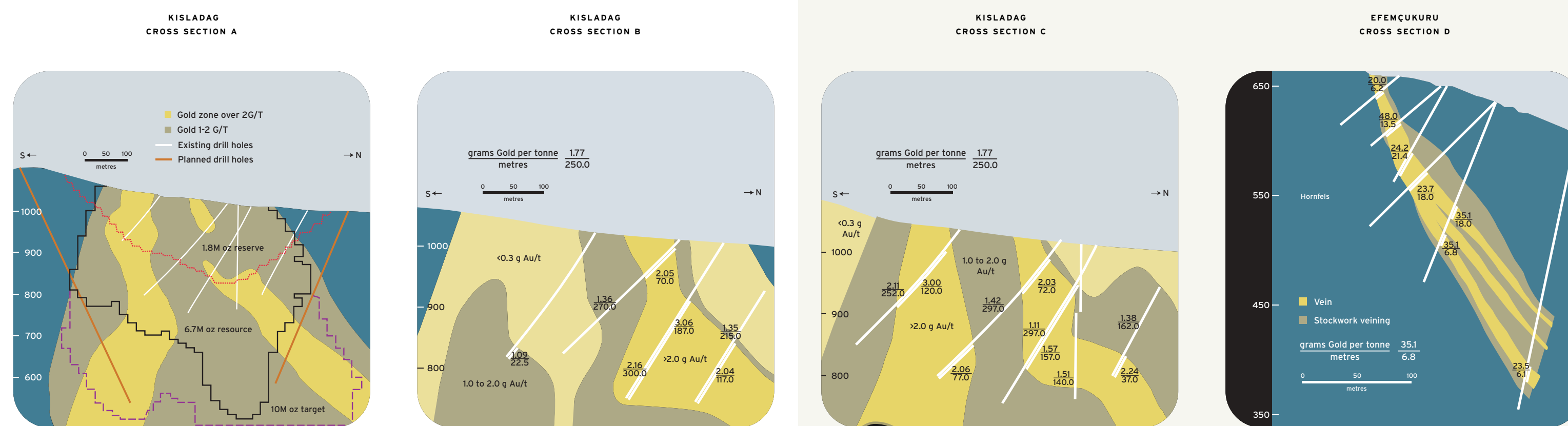
A drilling program at Kisladag (cross section A) will define the deposit boundaries and establish the validity of a larger target. We have identified higher-grade core mineralization at this site, forming in a zone that extends from the surface to drill-indicated depths of over 300 meters (cross section B). The porphyry-style deposit contains mineralization at various grades in concentric zones formed around a weakly mineralized intrusive (cross section C). At Efemçukuru, a well-defined high-grade epithermal vein structure hosts free-milling ore estimated to contain in excess of 1.1 million ounces of gold at 14 grams per tonne.
